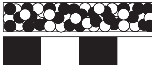
Figure 1. Spatially patterned catalyst bed; top: well mixed bed and bottom: layered arrangement; black: catalyst 1 and white: catalyst 2 (modified from Ref. 2).
